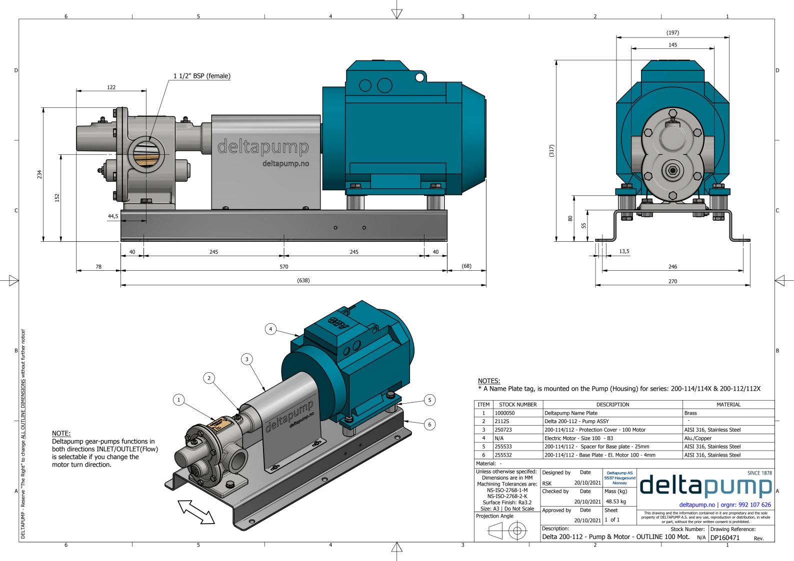
NOTE: This Pump, have an option to change Flow-direction to ease the install process. If a customer would like to change the direction of flow:
